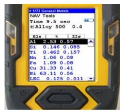
Perform light element analysis for Al alloys and specialty alloys without helium purge or vacuum.
